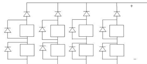
Connection of solar cells with diodes with bypass and blocking diodes
