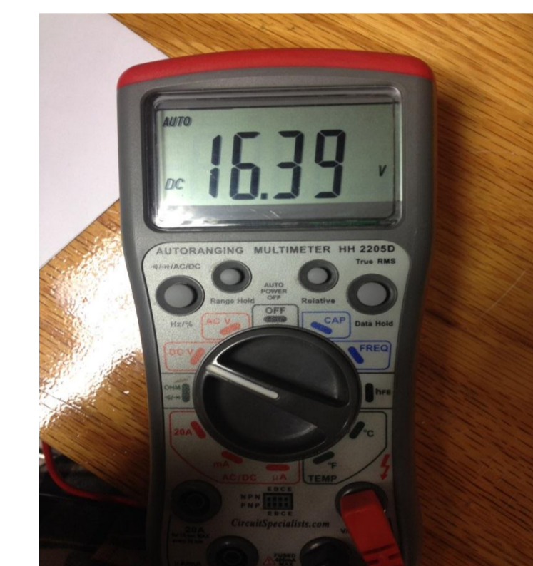
The voltage is rectified by the bridge rectifier.
