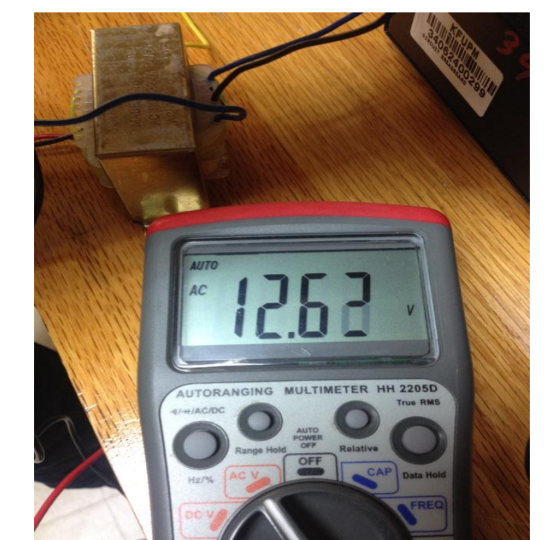
Transformer is used to step down the outlet voltage.
