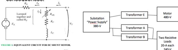
FIGURE 3: EQUIVALENT CIRCUIT FOR DC SHUNT MOTOR.
