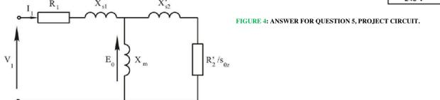
Figure 2: Equivalent circuit of the induction motor
