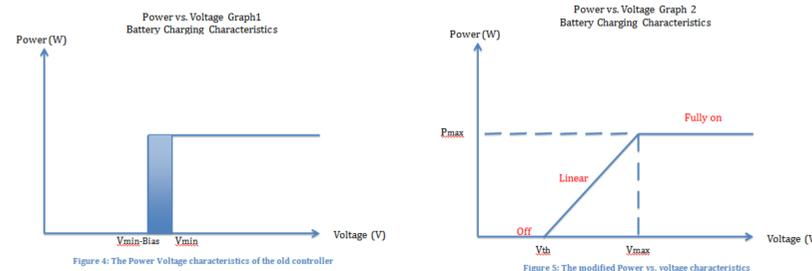
Figure 4: The Power Voltage characteristics of the old controller
