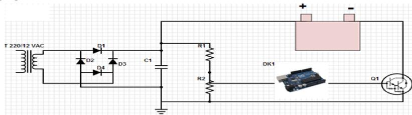
Figure 3: The controller unit circuit diagram
