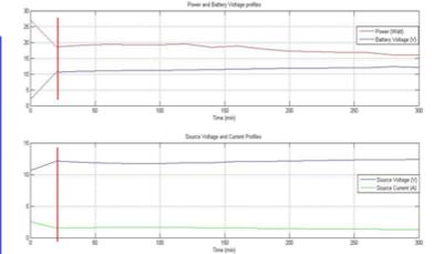
Figure 8: The Battery Charging Profile
