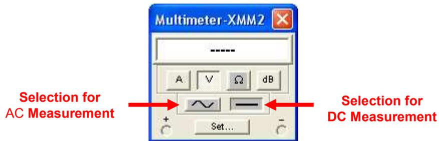
Figure. 15: **Multimeter** properties window
