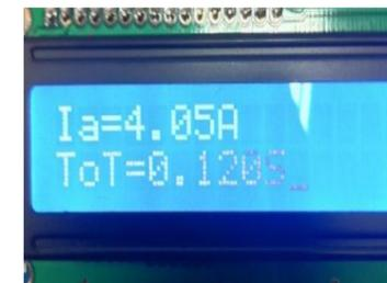
Fig.3: Tripping Time & Line Current on the LCD
