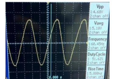
Fig.4: Conditioning Circuit Output in the Oscilloscope
