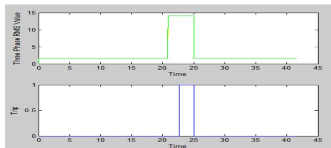
Fig. 2: Trip signal delay at fault condition.
