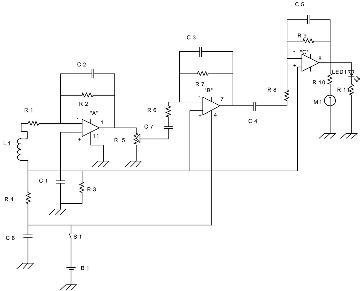
**Fig.1: Ferrous Motion Sensor Circuit Diagram ( A,B,C : 741 OA)**
