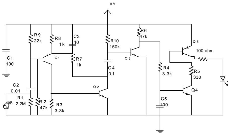
**Fig 3: Ultrasound Receiver Circuit**
