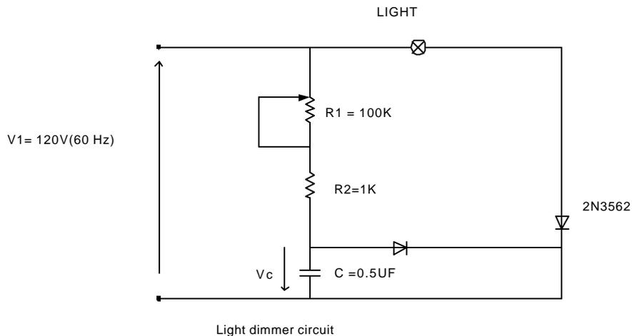
**Fig.1: Light Dimmer (or Motor Speed Control) Circuit**
