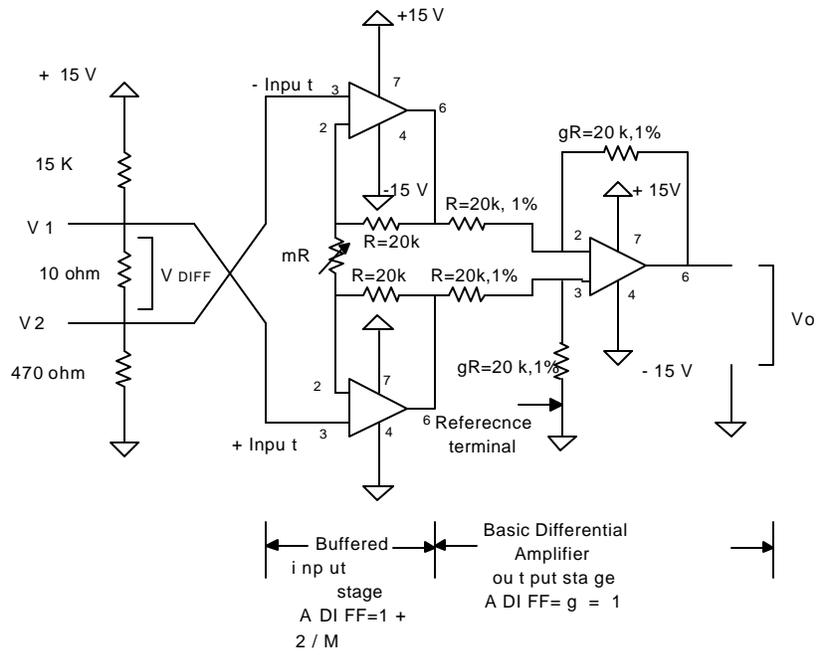
**Fig.3: Three Op-Amp Instrumentation Amplifier**
