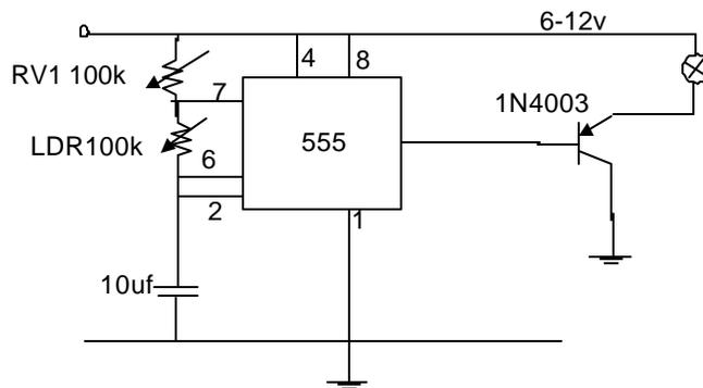
**Fig.3: Flasher Circuit**
