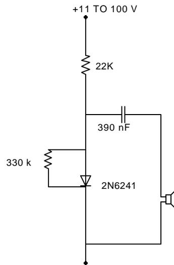
**Fig.7: Improved Circuit for Oscillations Generation**
