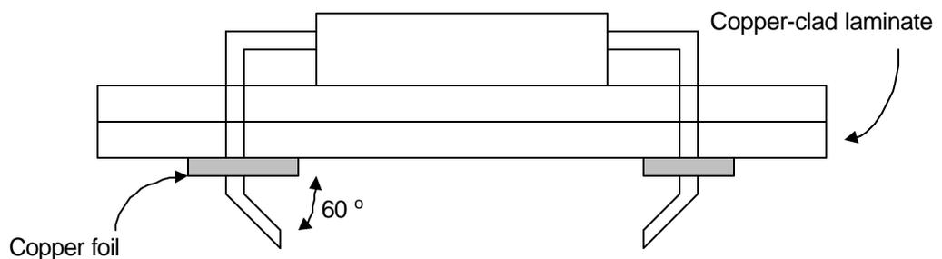
**Fig. 3: Components mounting**
