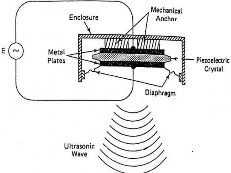
**Fig.1: Ultrasound Transmission (Schematic Diagram)**
